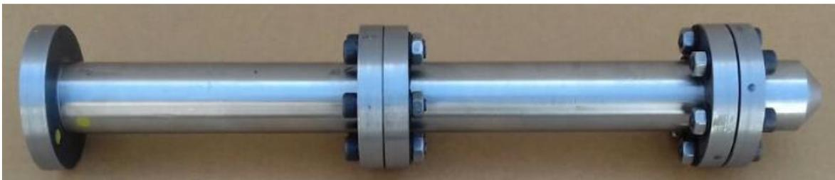
*Figura 4-7 Ensamble barril – boquilla extrusora*
